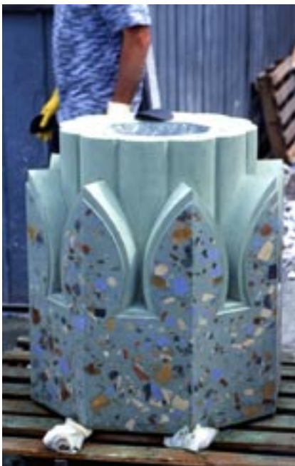
The hollow-cored 'Lotus' section, while in Diespeker's yard, being made by David Knowles. He was voted, by the Concrete Society, to be Britain's "Concrete Operative of the year 2000" )
